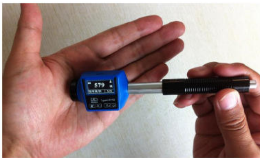
Leeb hardness measurement principle
